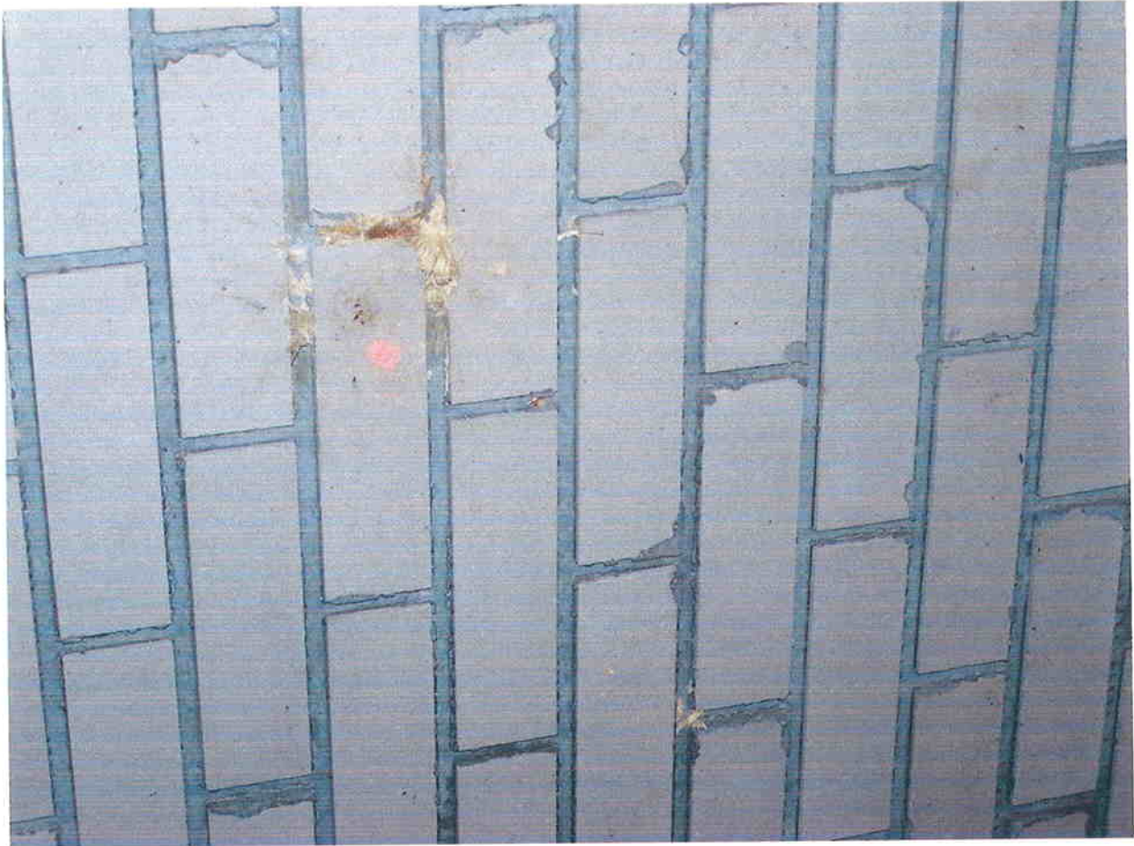
Missile III Imprint on Series 5, Specimen 1 8-in. panel face
