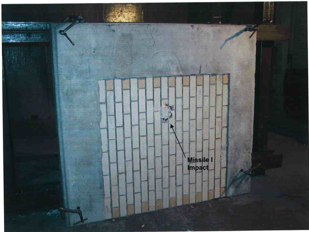
Missile Impact I of Series 3, Validation Specimen 2 Panel by DOE Pipe Projectile
