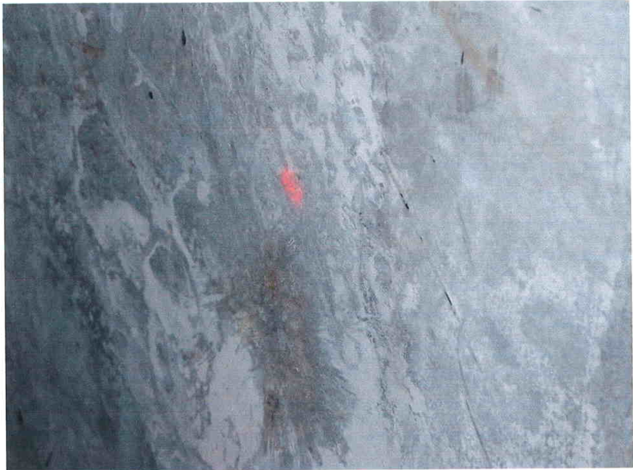
DOE Wood Missile Impact II of Series 1, Specimen 1 Panel
