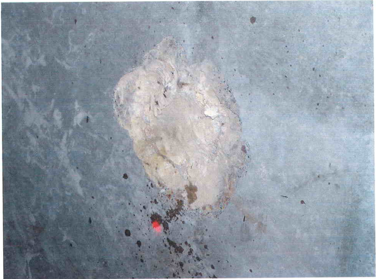
Missile IV imprint on Series 1, Specimen 1 Panel
