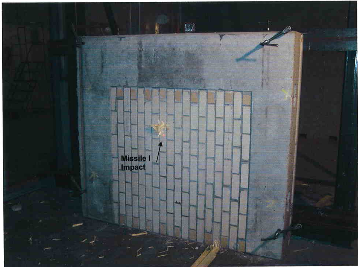
Missile Impact I of Series 5, Specimen 8-in. concrete side
