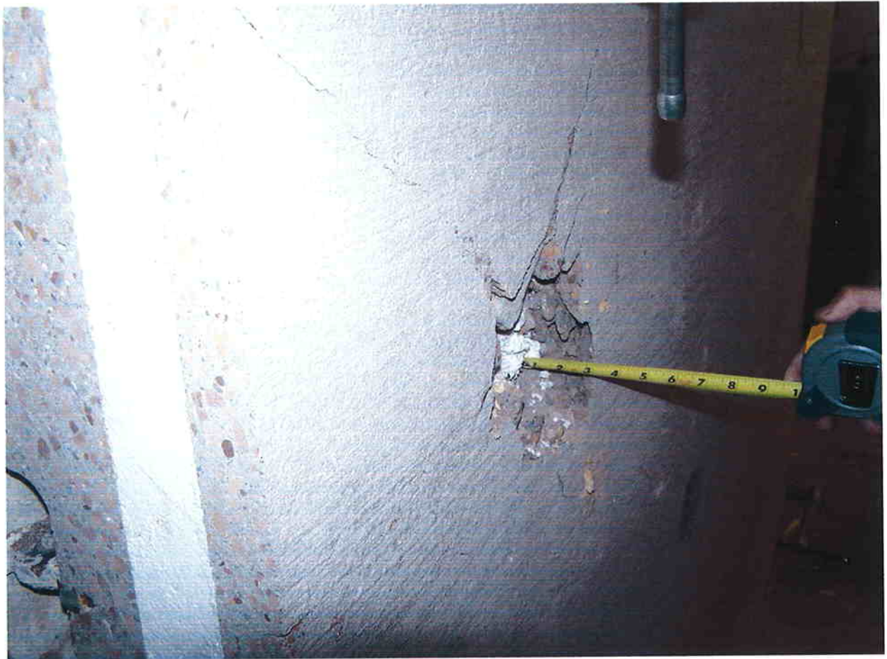
Series 5 Panel Penetrated 3-in. by Missile V
