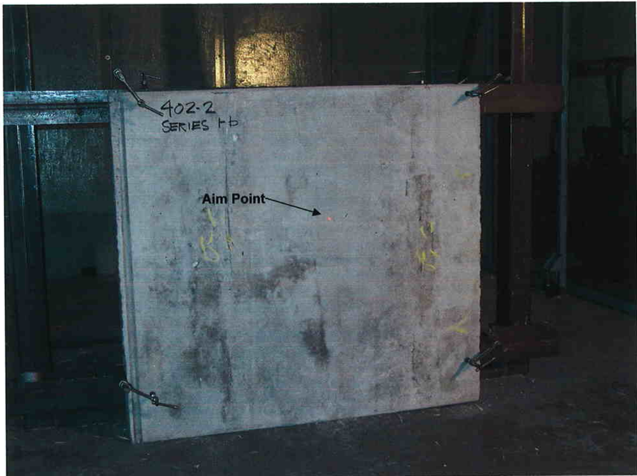
Series 1, Specimen 2 Panel erected for Doe Pipe Test
