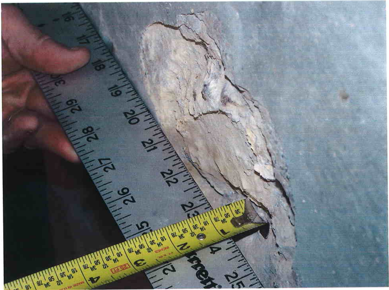
Missile Imprint Depth produced by DOE Pipe Missile IV
